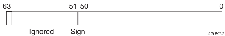
Figure 42. Fast operations with INTEGER(KIND=8) on CRAY T90 systems that support IEEE floating-point arithmetic
