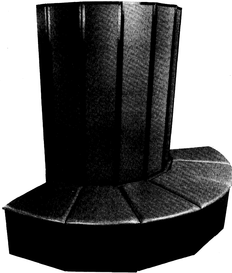
Figure 1-4. CRAY X-MP Model 22 or 24 6-column mainframe chassis
