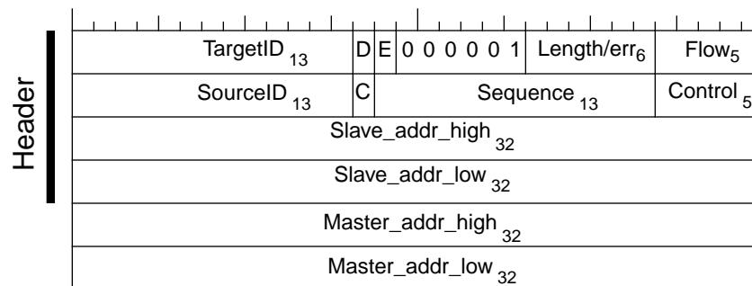
Figure 20. DMA Read Packet
