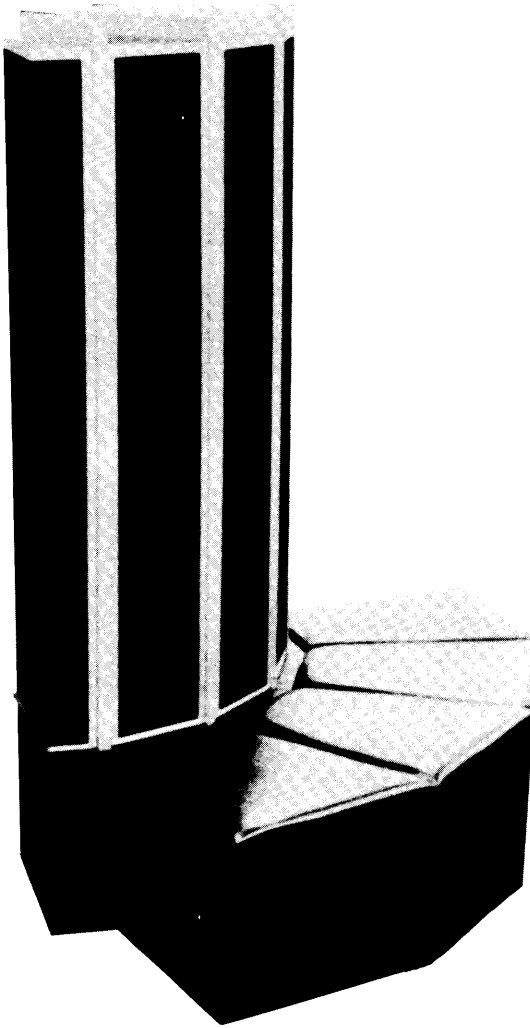
Figure 1-1. I/O Subsystem Chassis
