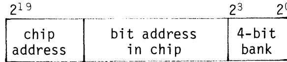
Figure 5-1. Memory address; 16 banks
