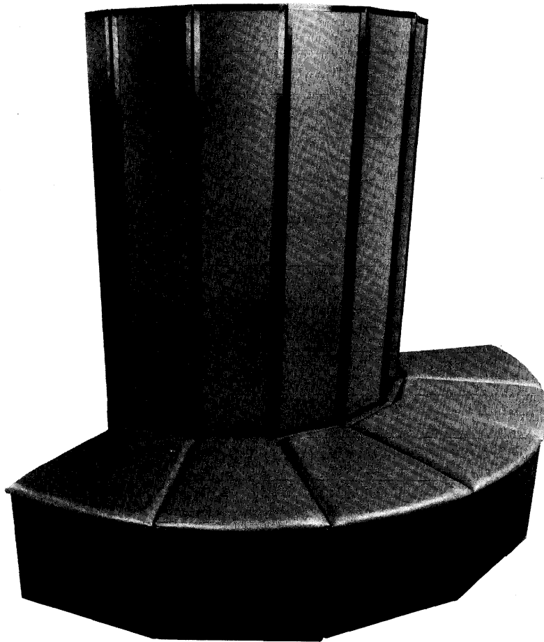
Figure 1-4. CRAY X-MP Model 22 or 24 6-column mainframe chassis
