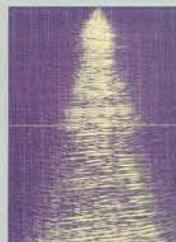
Common source seismic record after depth migration. It contains 96 traces, each six seconds long and sampled at an interval of four milliseconds, producing a total of 144,000 samples. Hundreds of these records are required to study subsurface geology. (Credit: Geo-Quest International, Inc.)
