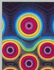
Charge density contours for an atomic overlayer of cesium on tungsten. Using a Cray system for computation and graphics generation, physicists have investigated the electronic structures of these materials and obtained results impossible to determine analytically. (Credit: Arthur J. Freeman, Henri J. F. Jansen, Erich Wimmer, Northwestern University.)
