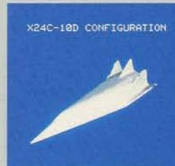
(Left) Full model of a Martin-Marietta X24C-10D Lifting Body. (Right) A transverse flow plane (perpendicular to the flight direction) just behind the cockpit. The coloration shows the variation in Mach number. (Far right) Flow plane at the tail of shuttle-like aircraft.
