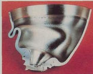
Experimental and computational results of the impact of a nose cone against an angled solid surface. (Left) Actual results and (right) the numerical simulation of this highly non-linear process. The striking similarity between the two confirms the validity of the computational approach. (Credit: Lawrence Livermore and Sandia National Laboratories.)
