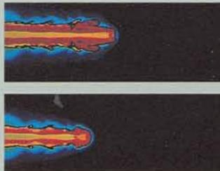
Evolutionary images of supersonic gas jets boring their way through other gases that are 100 times (left) and 10 times (right) denser. In simulating supersonic gas jets, the combination of color imaging with a Cray system enables one to probe in detail both the dynamics and internal physics of the gas flows. (Credit: Michael Norman, Larry Smarr and Karl-Heinz Winkler.)
