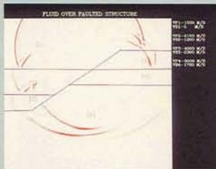
Color variable density displays of a seismic wave propagation from a fluid through a faulted structure. The full elastic equation was used, demonstrating the conversion of P waves (red) into S waves (blue). (Credit: Dan Kosloff and Moshe Reshet, University of Tel Aviv.)
