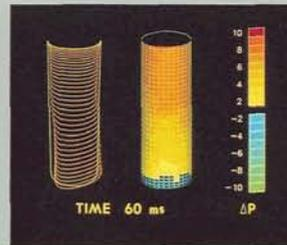
(Far left) A pressurized water nuclear reactor. The reactor core, primary and secondary heat exchange loops and containment system are shown. (Left) A cylindrical section of a nuclear reactor core with a calculated three-dimensional pressure field. The vertical color scale indicates the pressure drop ( $\Delta P$ ) in the vertical direction.
