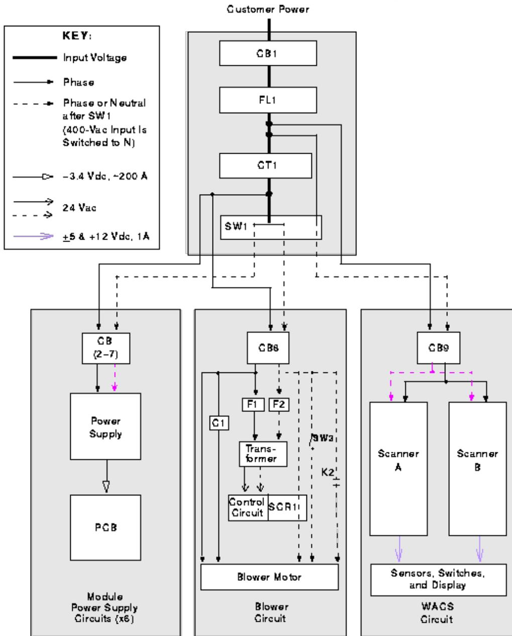
**NOTE:** Power also flows to the Clock Power Supply circuit breaker (CB10) in cabinet 0. CB10 controls power to the clock distribution power supply.
