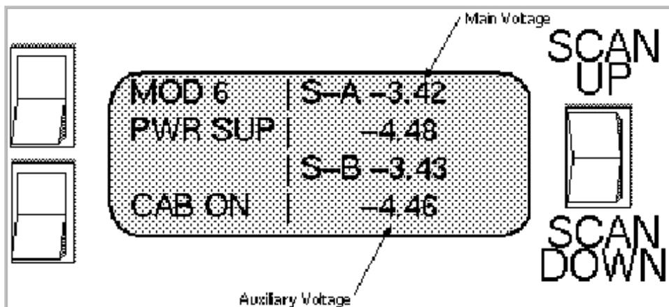
Table 14. Power Supply Screen Information - Clock Module Installed
