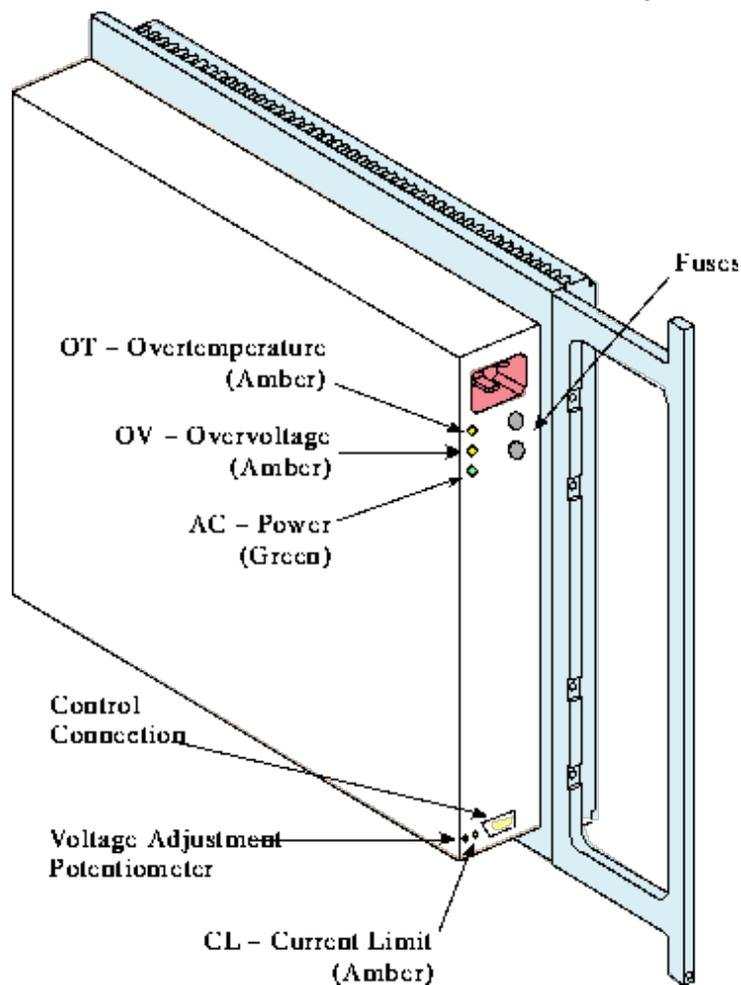
The power supply has four LED indicators, as shown in Figure 4.
