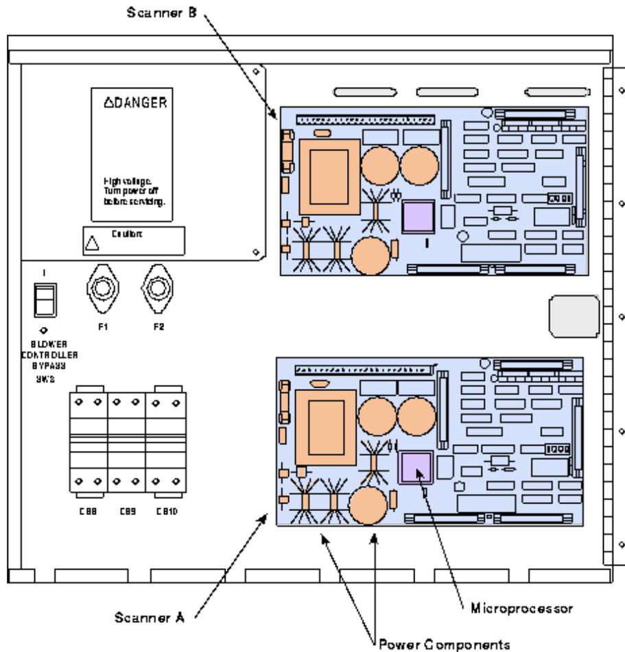
Each scanner contains a power connector strip (TB1) and five control connectors. The control connectors connect to the WACS wire harness. Each of the control connectors performs a primary function, as described in the following list:
