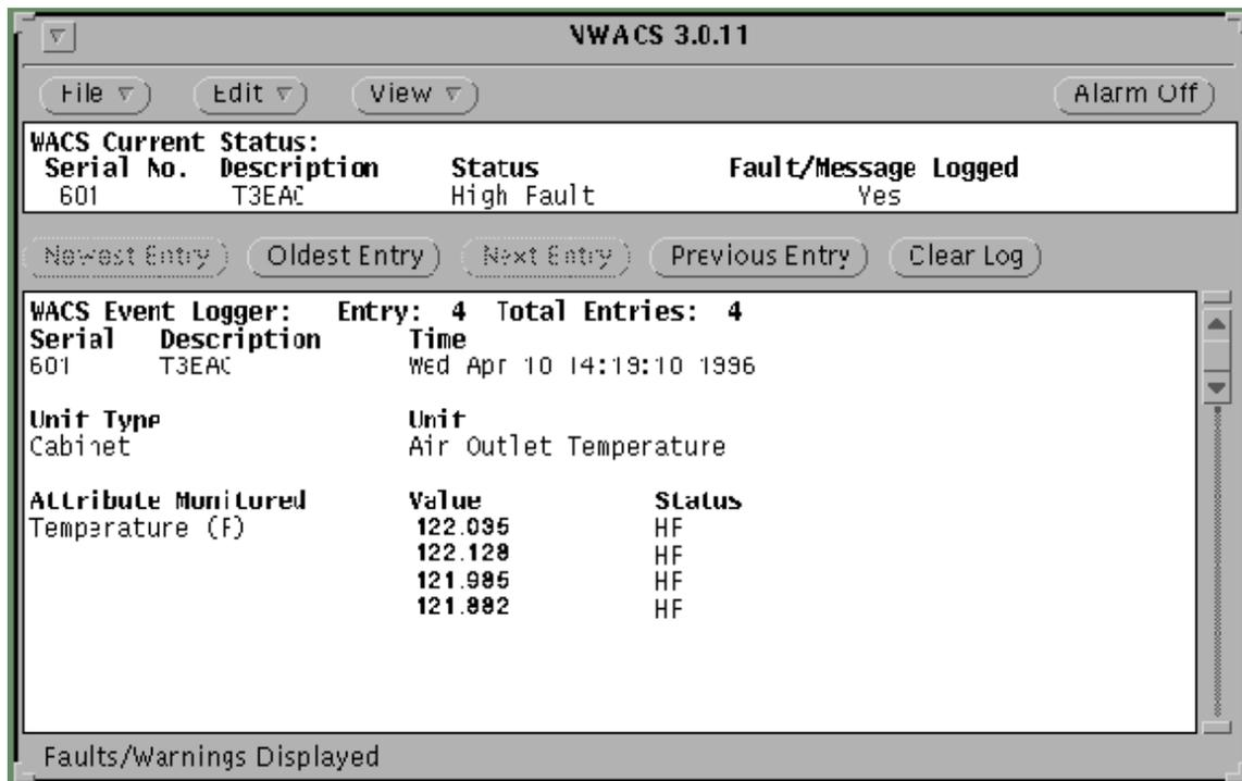
Figure 39 shows the main NWACS data screen. If NWACS records a fault, the associated text is shown in **bold** type.
