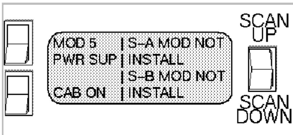
Table 12. Power Supply Screen Information - Module Not Installed
