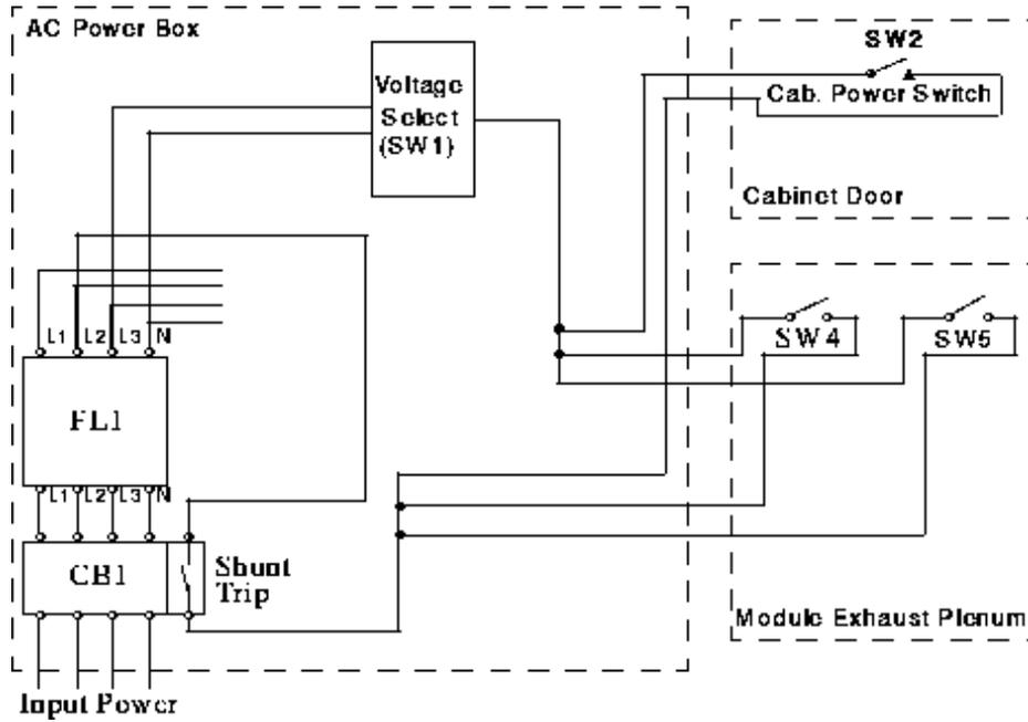
Figure 13. Cabinet Power Switch (SW2) - Location
