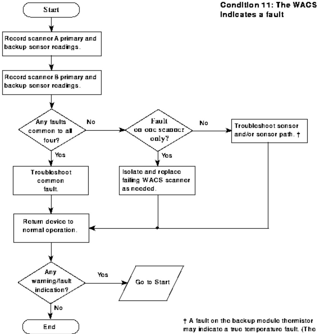
† A fault on the backup module thermistor may indicate a true temperature fault. (The temperature of the backup module thermistor is usually higher than the temperature of the primary module thermistor.)
