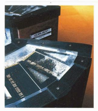
Technological innovations on the CRAY-2 include the use of liquid immersion cooling and the eight-layer, three-dimensional modules.
