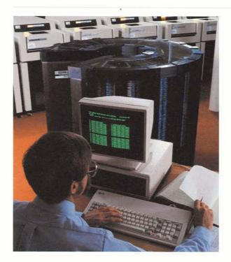
Control of network access equipment and the high-speed disk drives is integral to the CRAY-2 mainframe hardware. A single Foreground Processor coordinates the data flow between the system Common Memory and all external devices across four high-speed I/O channels. The synchronous operation of the Foreground Processor with the four Background Processors and the external devices provides a significant increase in data throughput.
