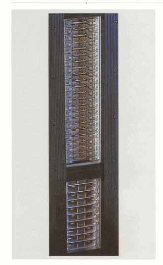
The CRAY-2 mainframe is elegant in appearance as well as in architecture. The memory, computer logic and DC power supplies are integrated into a compact mainframe composed of 14 vertical columns arranged in a 300° arc.
